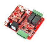
The modules allow you to enter the values of two digital signals from 9V to 300V both DC and AC. Compliant to IEC 61131-2; Type 1, 2, 3 characteristics for 24-V isolated digital inputs. Accurate Current Limit for Low-Power Dissipation – 2.2 mA to 2.47 mA for Type 3. The maximum insulation voltage (up to 60 s) is  $3600V_{PK}$ .
