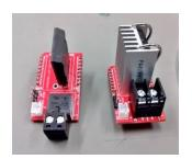
**BOKRA 60VDC SSR xx** modules contains IXYS SSR (Solid State Relay) CPC1709. There are two versions of the module, with a different output connector:
