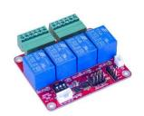
The **BOKRA I2C 4RO SRD** module has four <u>SRD-05VDC-SL-C</u> relays. Rated resistive load: 7A at a voltage of 240 VAC or 28 VDC. Contact form - SPDT. The galvanic isolation is individual. The dielectric strength of the insulation is 1,5 kV AC (for one minute between the coil and the contacts) and 1 kV AC (for one minute between the contacts of the same polarity).
