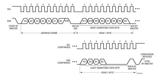
Due to that, before any further processing, the 16-bit value received from LTC2309 must be shifted to the right for 4 bits. The result value is  $X_{ADC.}$
