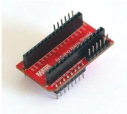
The **Arduino Nano Shield** is an adapter that allows you to install Arduino Nano compatible modules in the mikroBUS slot or connect mikroBUS modules (such as [MikroElektronika's Click®](#)) to Arduino Nano or compatible modules.
