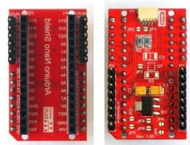
**Arduino Nano Shield** size - 43.18 x 25.4 mm.
