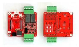
Input Power: 9-36VDC. The DC-DC converter produces uninsulated power 5VDC, 1,5A. Overvoltage and reverse polarity protection.
